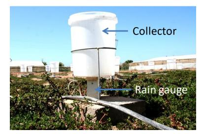
**Figure 4.** Collector attached to each automatic rain gauge
