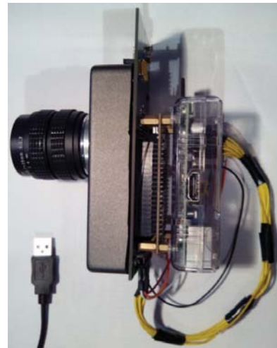
Fig. 3. Photograph of the chip with the carrier board, the lens, and the FPGA for control signals.
