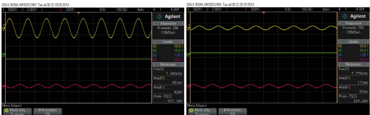
Figure 14: Experimental oscillations with the AGC. (a) 100% occupation level. (b) 10% occupation level.
