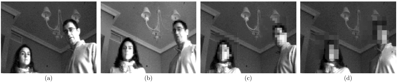
Figure 5: On-chip obfuscation without artifacts: (a) Original image captured by the chip. (b) Pixelation with 4 \times 4 -px blocks. (c) Pixelation with 8 \times 8 -px blocks. (d) Pixelation with 16 \times 16 -px blocks.
