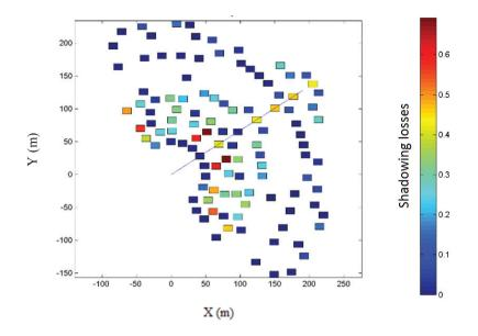
Fig 3. Optimized variant of the 113 heliostat field, 4pm. Colors represent shadowing loses.
