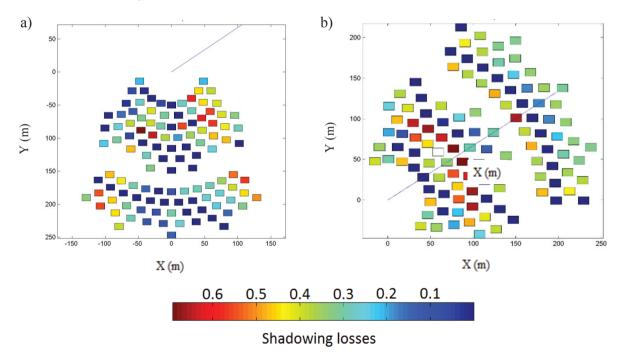
Fig 2. (a) Fixed variant of the 113 heliostat field, 4pm. (b) Rotating variant of chosen field, 4pm. Colors represent shadowing loses.
