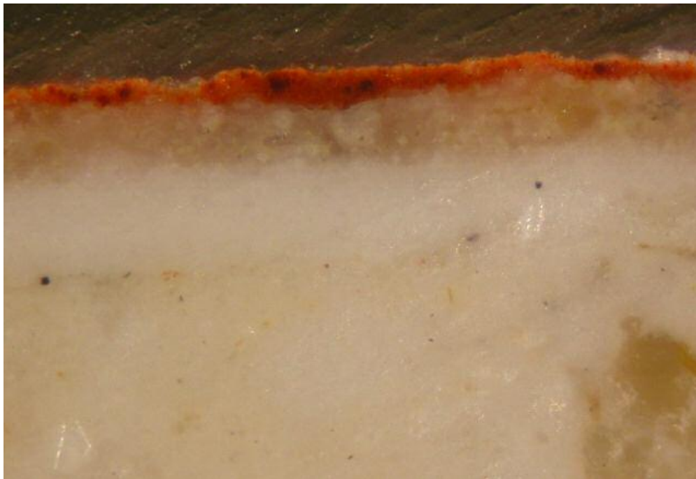
Selected optical micrograph of cross-section sample of mural painting in Crngrob showing the combination of lime technique and painting on a dry surface (a secco).
