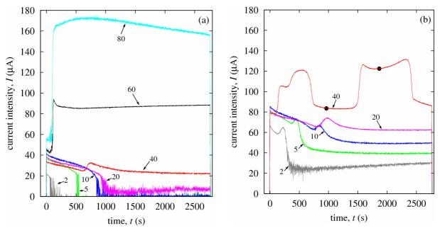
Fig. 1: Time evolution of corona current intensity in mixtures of  $CO_2$  and  $N_2$  for (a) V = 7 kV and (b) V = 8 kV. The volume percentage of  $N_2$  corresponding to each line is indicated in the figure.
