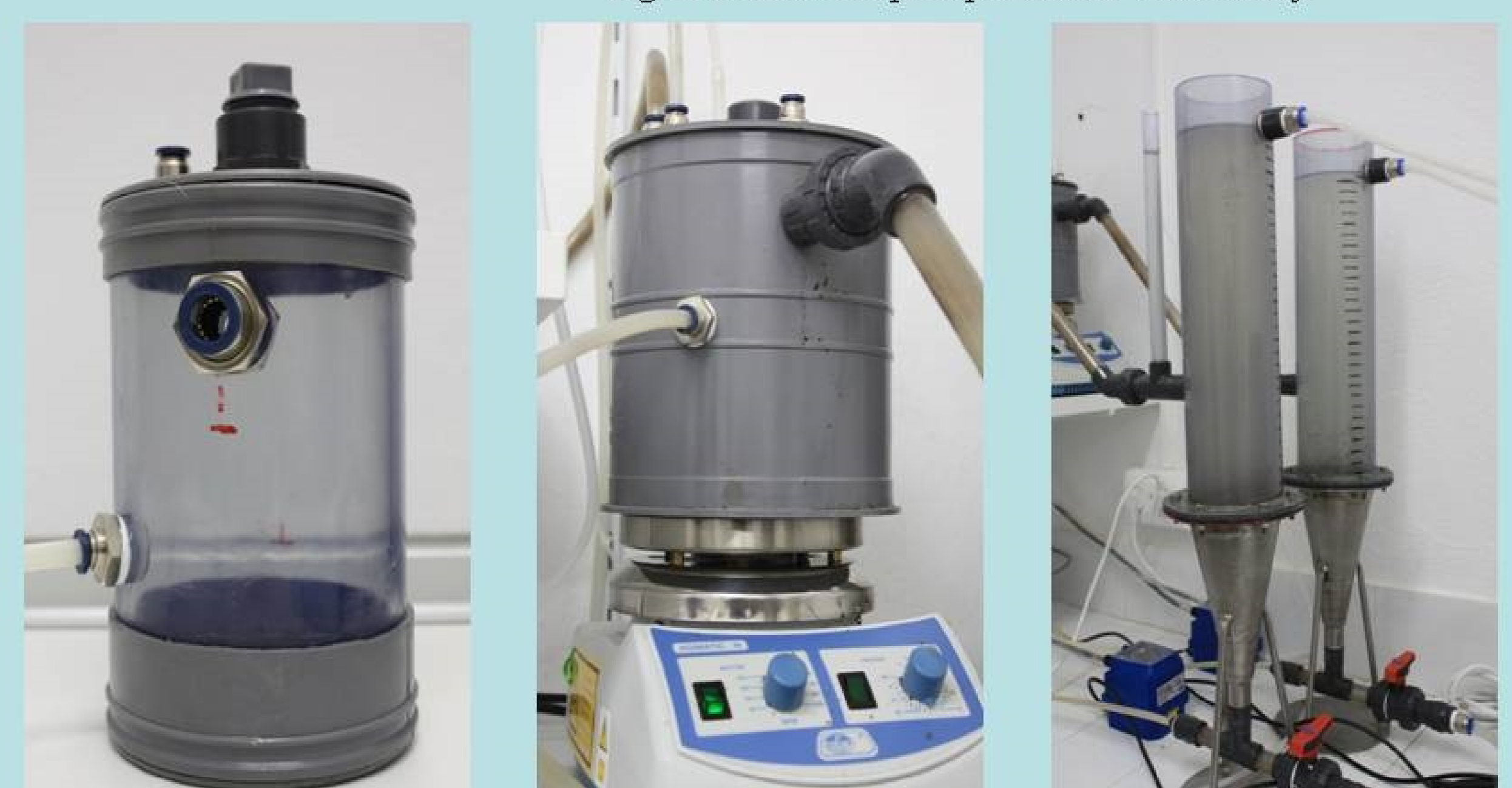
Figure 3. Detail of the two pilot plants. Anoxic tank, aerobic tank and settler.
