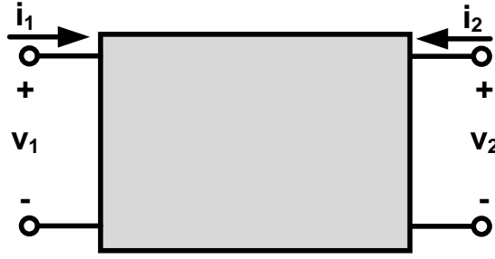
Figure 4.1: Two-port representation of an operational amplifier.
