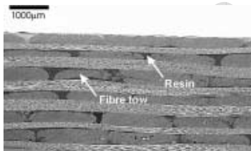
Figure 1. Cross-section of a typical NCF composite [2].
