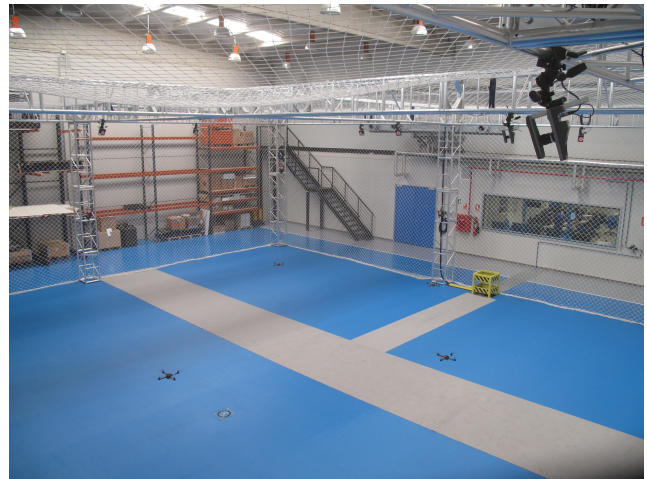
Figure 10. Indoor multi-UAV testbed of the CATEC with Hummingbird quadrotor from Ascending technologies.
