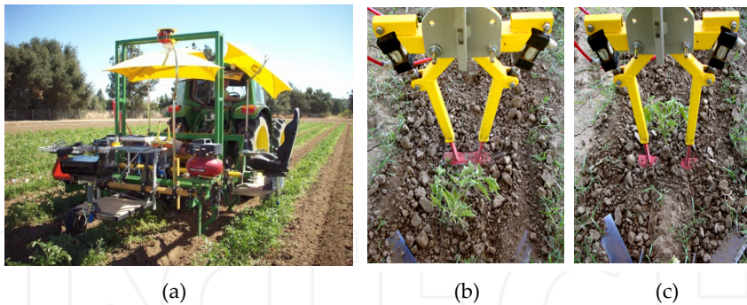
Figure 16. A RTK-GPS based robotic cultivation system-(a) A cultivator retrofitted with a RTK-GPS system in operation, and (b) The cultivating tines open to protect the plant based on the plant map and closed to get rid of weeds in between plants in the crop row.
