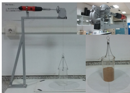
Figure 2. Lab equipment for determining the angle of repose.
