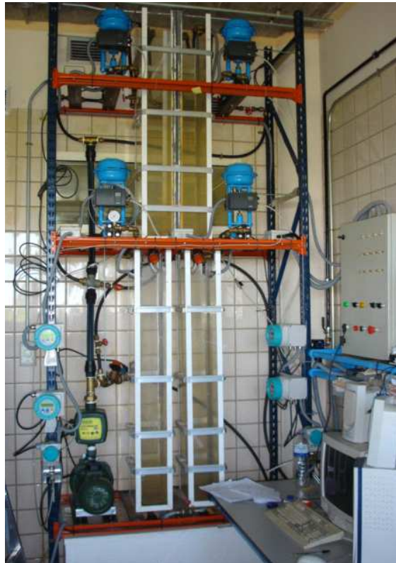
Figure 2.19: A photo of the four tank plant
