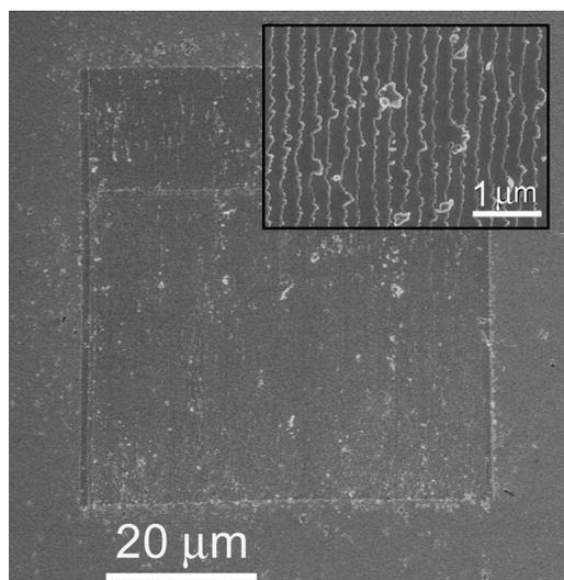
FIG. 1. SEM image of a  $\sim 60 \mu\text{m} \times 60 \mu\text{m}$  square pattern obtained by nano-scratching a 2000 nm thick crystalline  $\text{Ge}_2\text{Sb}_2\text{Te}_5$  film with a force of  $300 \mu\text{N}$ . In the inset a higher magnification image of the scratches. Scratches have a width of  $\sim 500$  nm and are separated by 250 nm one from the other, so that no area within the square pattern is left unmodified.
