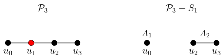
Figure 2.3: A cut set S_1 = \{u_1\} of \mathcal{P}_3 and the components of \mathcal{P}_3 - S_1 .
