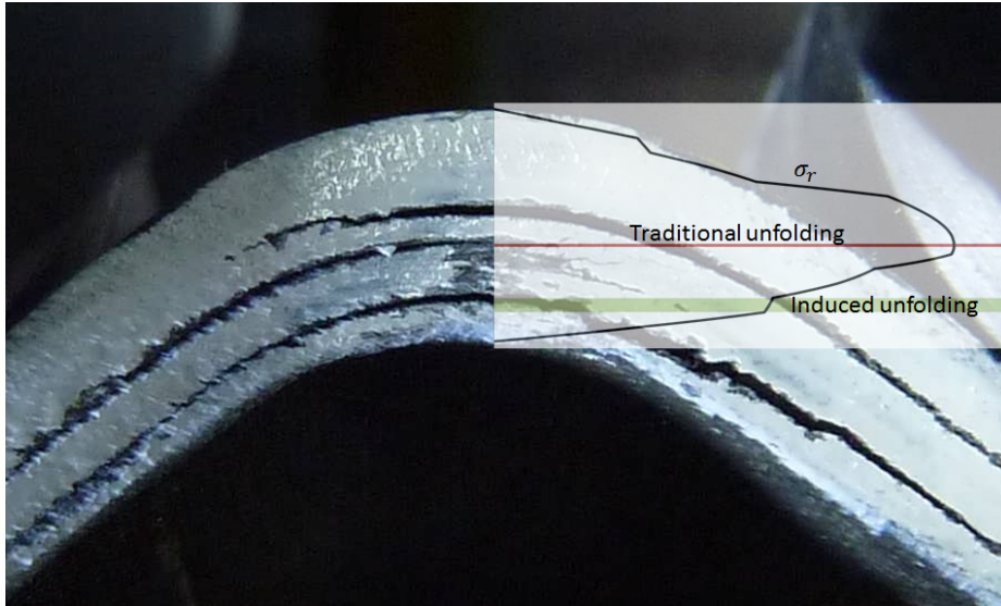
Figure 5.6: Location of the delaminations in a CP2/CP3 coupon.
