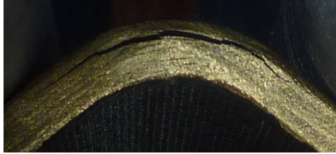
Figure 5.2: Induced unfolding initiated by a fibre compressive failure.
