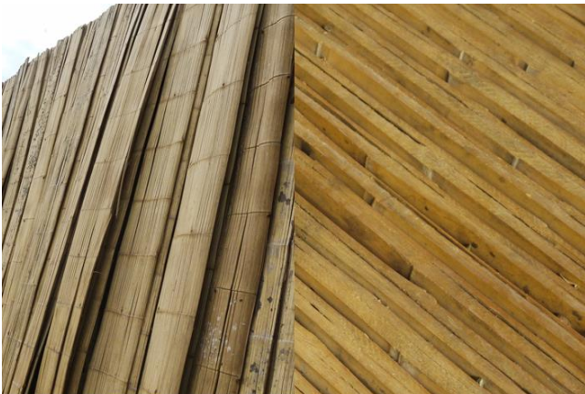
Fig. 2 Mats (left) and cans (right) of guadua. Source: Photo by José E. Torres R.
