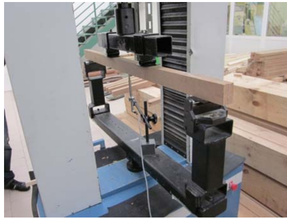
Fig. 4 MDF duo beams tested according to UNE EN-408.
