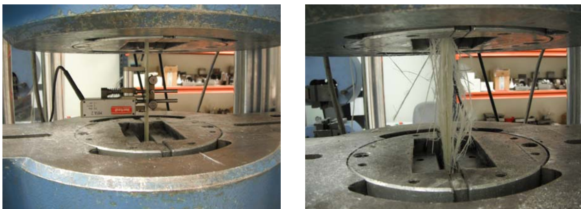
Fig. 3 Tensile test according to ISO 527-5 of the rigid bands GFRP.
