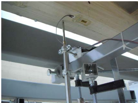
Fig. 9 Monitoring and loading of creep tests.
