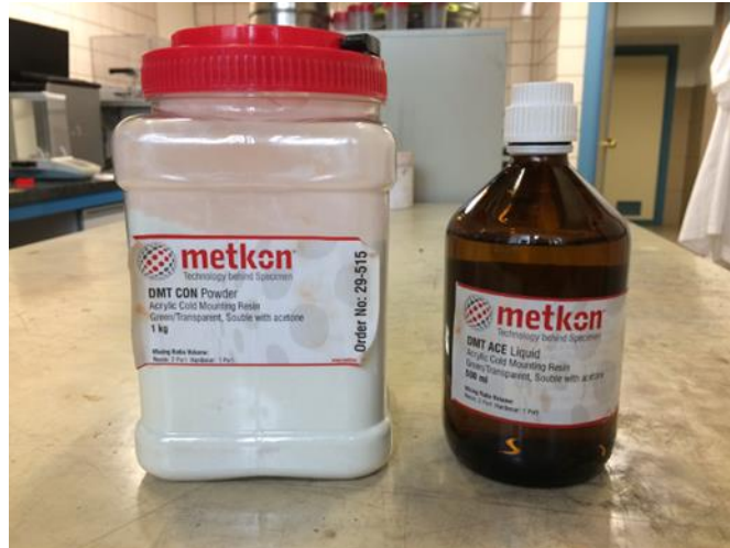
Figura 62. Resina Acrylic Cold Mounting Resin , Metkon ( Technology behind Specimen ).
