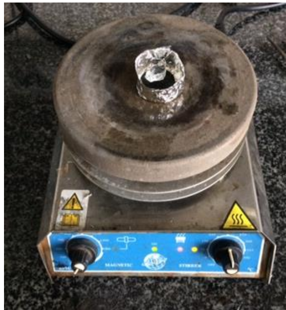
Figura 61. Placa calefactora para poner la resina QuickStick™ 135 Mounting Wax ( South Bay Technology Inc., San Clemente, CA, USA ).
