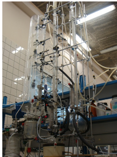
Fig. 1. A 0.48 kg CO 2 /h lab-scale CO 2 capture rig.
