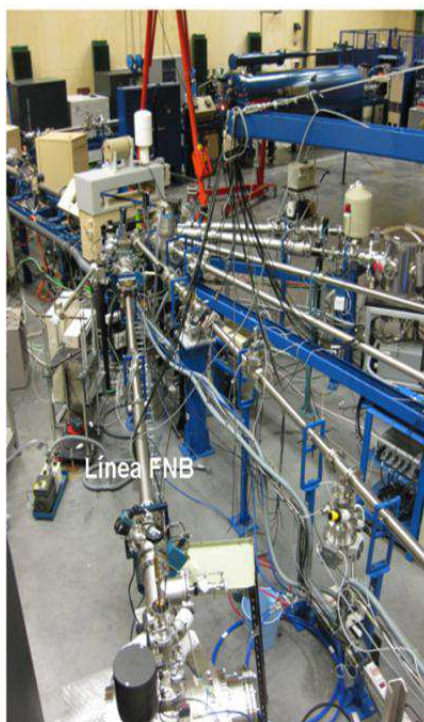
FIGURE 4.6: Top view of the seven beam lines coming out from the 3MV Tandem accelerator at CNA
