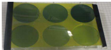
FIGURE 4.11: EBT3 film showing circles irradiated with six different dose values
