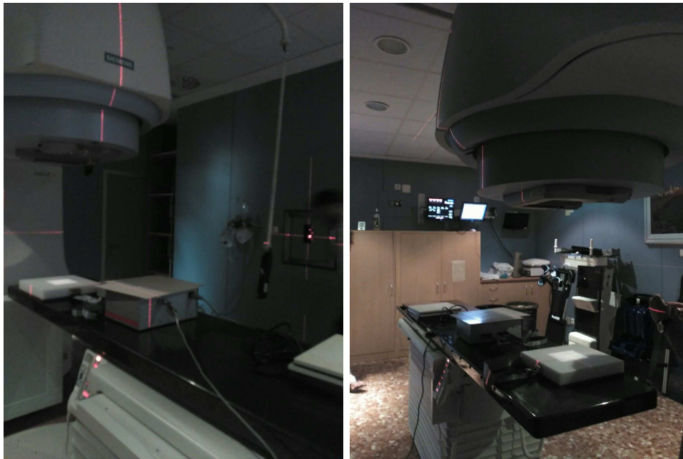
FIGURE 3.4: Experimental setup used for the measurements: both pictures show the linac head, the slab phantom centered with the laser system of the clinical treatment room, and the electronics.
