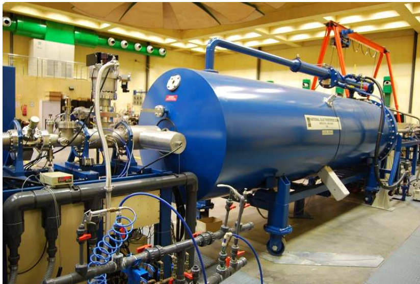
FIGURE 4.5: Picture of the 3 MV Tandem Accelerator at the CNA
