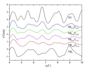
**Figure 3.**  $k^2$ -weighted EXAFS,  $k^2\chi(k)$ , of TiBC/a-C samples as a function of the photoelectron wave number k, together with fcc-TiC and h-TiB<sub>2</sub> standards.
