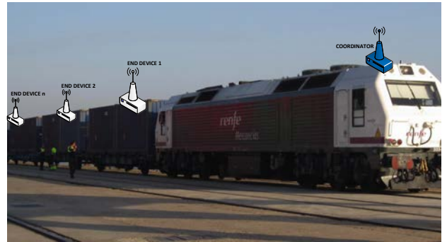
b) Network deployed in a cargo train
