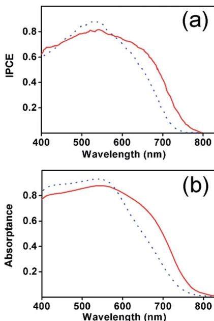
Fig. 1 (a) Experimental IPCE as reported by Arakawa *et al.* in ref. 13 and (b) calculated optical absorbance as estimated with the theoretical model herein proposed. In our model, we use as input parameters the data reported in their manuscript (electrode thickness of 17.5 microns, 40 vol% particle concentration, and 100 nm diameter).
