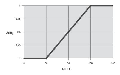
Fig. 1. Utility example for Mean Time To Failure
