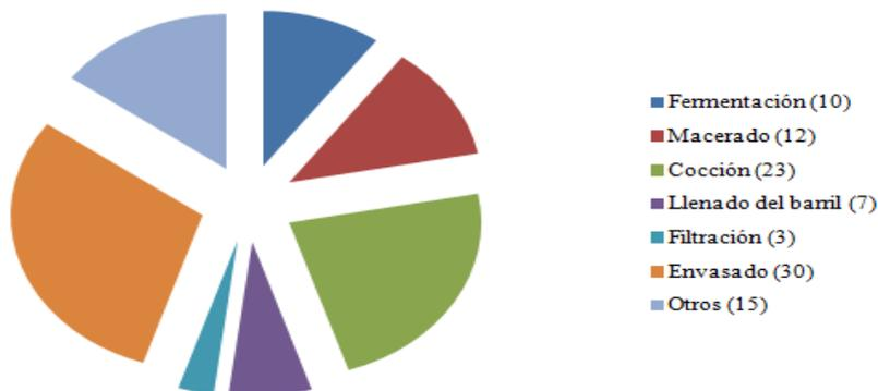
Figura 2-19 Demanda de calor y frio (térmica)en una cervecería(%). Fuente: Systems supporting production engineering, Review of problems and solutions, 2015, No.1(10).
