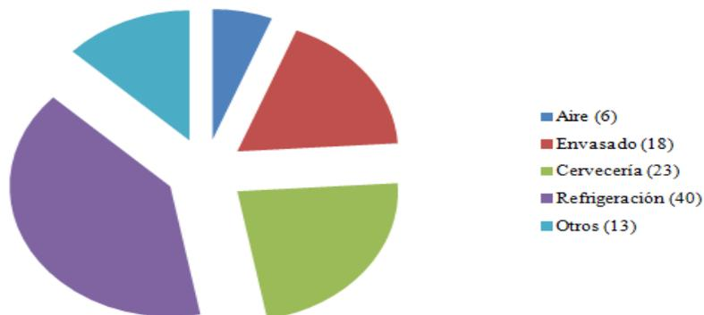
Figura 2-18 Demanda eléctrica de una cervecería(%). Fuente: Systems supporting production engineering, Review of problems and solutions, 2015, No.1(10).
