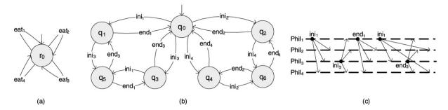
Fig. 1. (a) A four-philosopher system in which each *eat* transition co-ordinates a philosopher with its two neighbouring forks. (b) A refined system in which the *ini* and *end* transitions represent the start and finish of the corresponding *eat* actions. (c) Part of a concurrent execution with conflicting observations.
