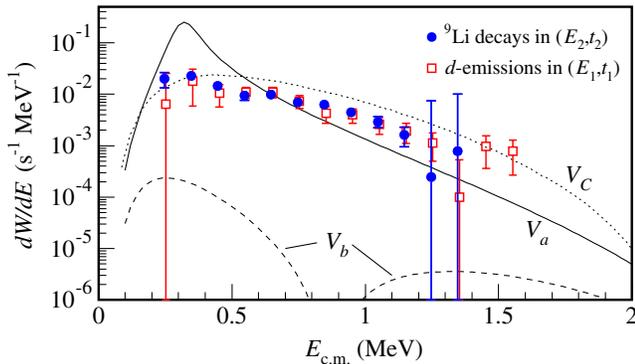
FIG. 3 (color online). Transition probability for the  $^{11}\text{Li} \rightarrow ^9\text{Li} + d$  decay channel. The procedures to obtain the experimental data are explained in the text. The curves are predictions from Refs. [7] ( $V_C$ ) and [8] ( $V_a$  and  $V_b$ ).
