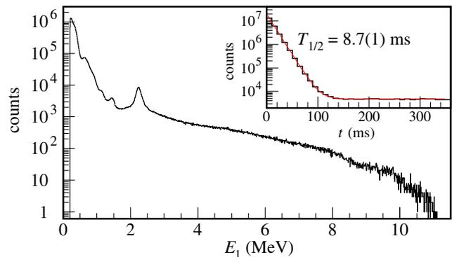
FIG. 1 (color online). Energy spectrum of ( $E_1, t_1$ ) events, defined as those following a  $^{11}\text{Li}$  implantation in the same pixel within 40 ms: These are  $^{11}\text{Li}$  decays. The inset shows the time behavior of all events following an implantation: The short-time component has the expected  $^{11}\text{Li}$  half-life.
