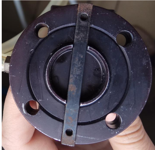
Figura 47: Detalle cogida pinza angular Cleveland Guest Engineering LTD.
