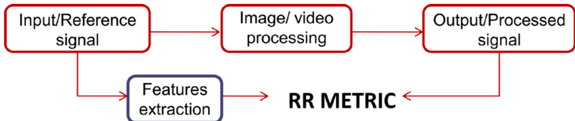
Figura 2: Diagrama de métodos Reduced Reference
