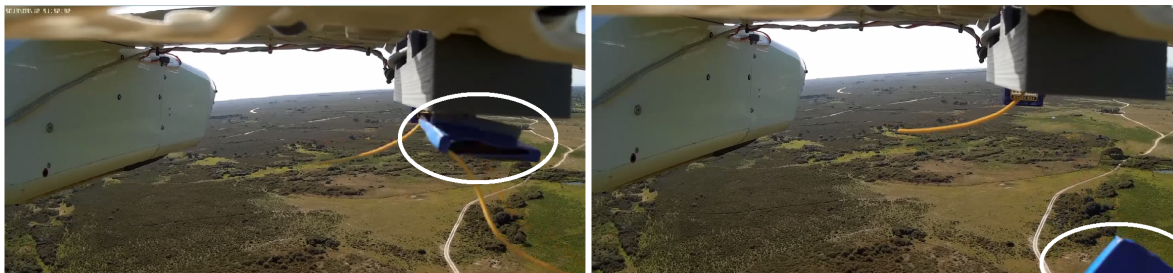
Figure 5. Pictures taken during the activation of the sensor node deployment mechanism. The sensor node protected with a blue color enclosure is marked in the images.
