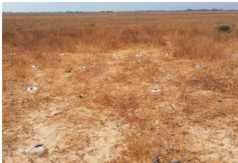
Figure 2. Some TelosB WSN nodes deployed in the field experiments. For better visualization in the picture, the nodes were put on top of plastic boxes.
