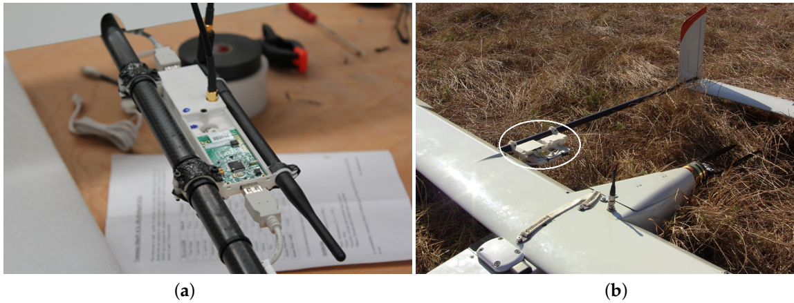
Figure 4. Pictures of the TelosB node on board the UAS: (a) detail and; (b) mounted on the UAS.
