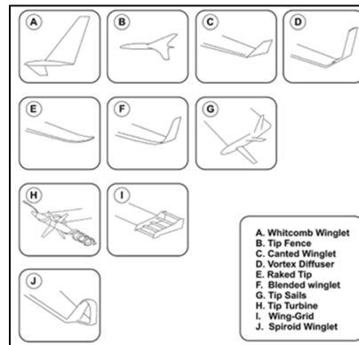
Fig 2. Various winglet solutions.
