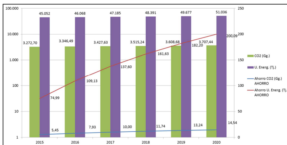
Fig 6 Evolution of CO 2 emissions, energy units and their saving for the period 2015-2020. Optimistic scenario.
