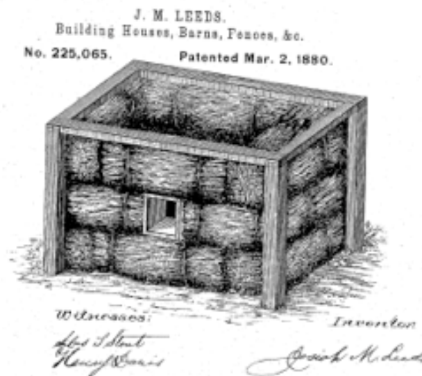
Fig.2 "US Patent 225 065 A, in March 1880, Straw Bale Building" Source: https://encrypted.google.com/patents/US225065
