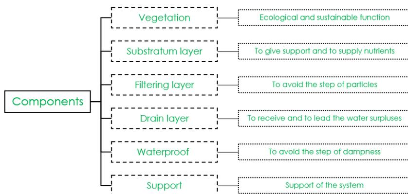
Fig. 1 "Green-roof system components". Reference: García, I. México, 2011.
