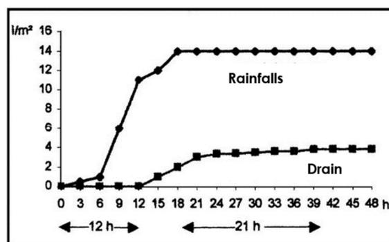
Fig. 3 "Volume of rainfall and storm drain in an green-roof after a continuous rain of 18". Reference: Minke, G. Cuba, 2014
