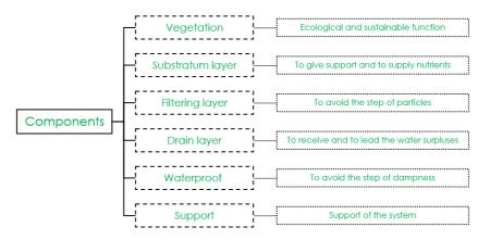
Fig. 1 "Green-roof system components". Reference: García, I. México, 2011.
