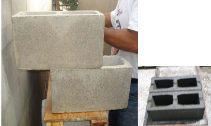
Figure 3 shows on the left side a commercial cemented block and on the right side a cemented diathermic block.
