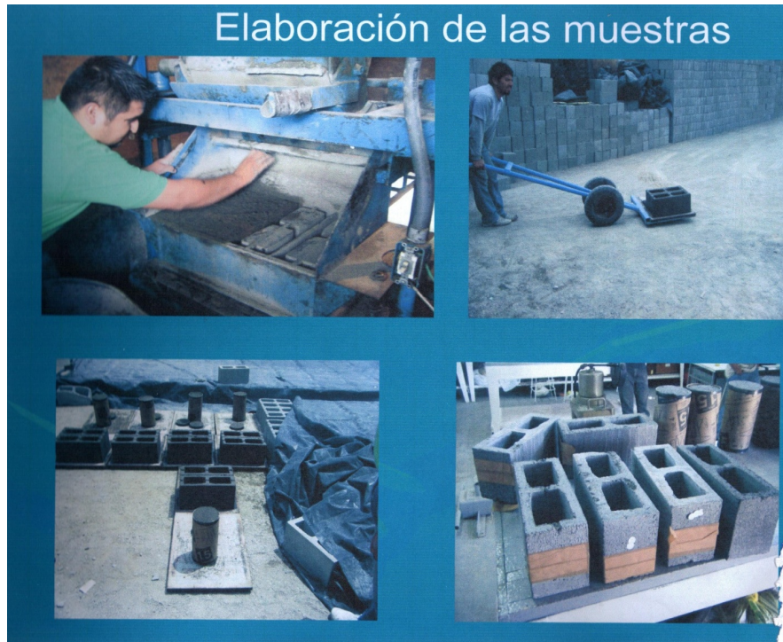
Fig. 2 Elaboration of samples of the cemented diathermic block.
