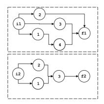
Fig. 4. Two sample projects on activity on node notation
