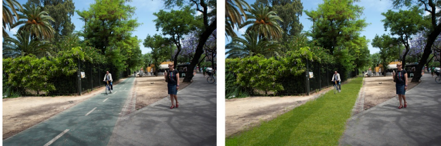
Fig. 6 Hypothetical bike path formed by a permeable continuous surface of artificial grass consisting of an industrial carpet manufactured with plastic and synthetic materials, specifically polypropylene fibers with high recyclability and water collection system
