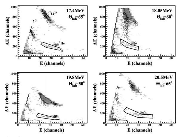
FIG. 1.  ${}^{6}\text{He} + {}^{120}\text{Sn}$  biparameteric spectra. The  $\alpha$ -particle group is shown inside the poligon and the peak above corresponds to the  ${}^{6}\text{He} + {}^{120}\text{Sn}$  elastic scattering
