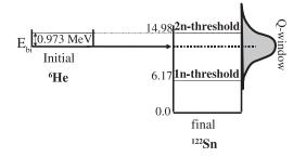
FIG. 3. Scheme showing the excitation energy region populated by the 2*n* transfer leading to the <sup>122</sup>Sn nucleus. The separation energies  $S_{1n}$  and  $S_{2n}$  for the <sup>122</sup>Sn nucleus are indicated in MeV.
