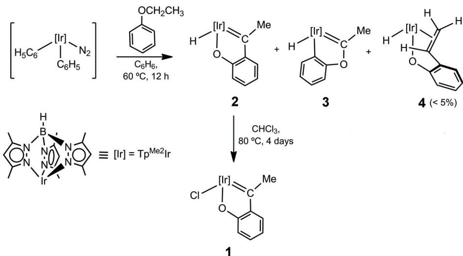
**Figure 3**Reaction scheme for the synthesis of **1**.
