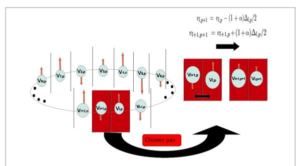
**Figure 1.** The model is defined on a lattice, each site being characterized by a velocity  $v_l$  and standing for a fluid slab. The dynamics proceeds via nearest-neighbour collisions as defined in the text, in which part of the energy is dissipated. This model resembles a sheared granular system at the mesoscopic level. To be specific, we show the sketch that corresponds to periodic boundary conditions.
