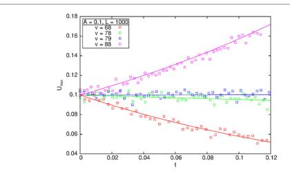
**Figure 2.** Rescaled velocity profile maximum  $U_{\text{max}} = U(x_M, t)$  as a function of time, where  $x_M = 1/4$ . Trajectories start from a sinusoidal average velocity profile  $u(x, 0) = u_0 \sin(2\pi x)$  (here  $u_0 = 0.1$ ), which gives hydrodynamic predictions  $U(x, t) = u_0 \sin(2\pi x) e^{(\nu - \nu_c)t/2}$  (drawn as solid lines).
