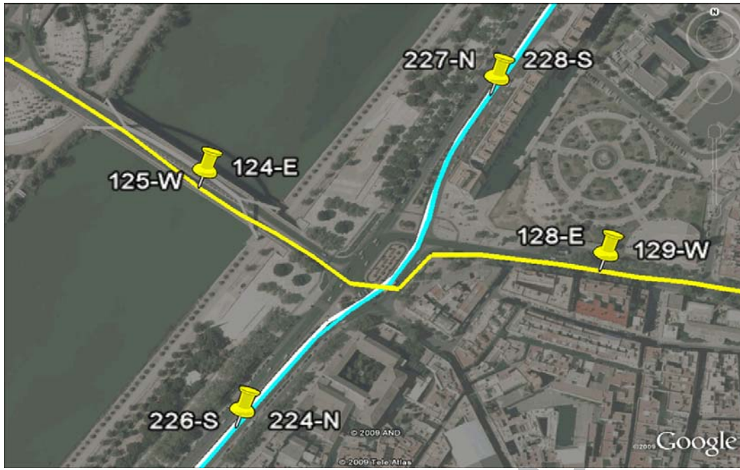
Figure 2. Support points generated in a real situation: Each support point is far enough from the crossroads to prevent the GPS device from indicating an erroneous significant observation. The same point can be traversed in different directions and hence the system labels each one with the possible directions of the trip.
