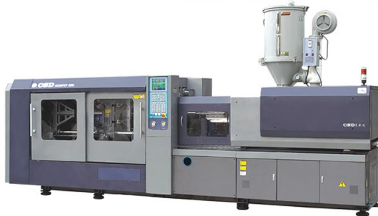
**Figure 1.15. View of an injection molding machine<sup>9</sup>**
