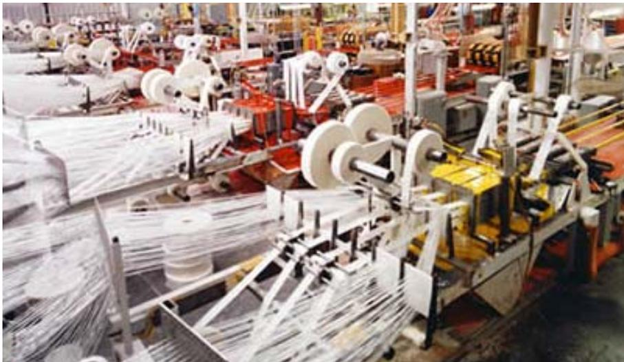
**Figure 1.11. View of a pultrusion machine<sup>6</sup>**
