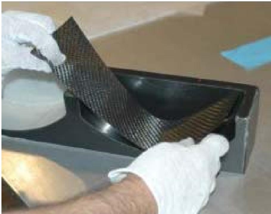
**Figure 1.6. View of a stage of the hand lay-up process<sup>4</sup>**
