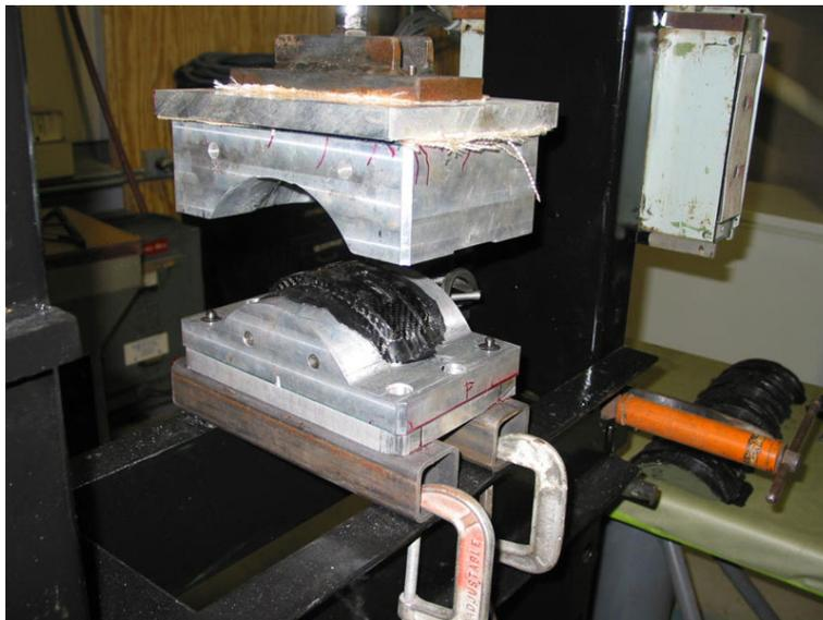
**Figure 1.13. View of a compression moulding machine<sup>8</sup>**
