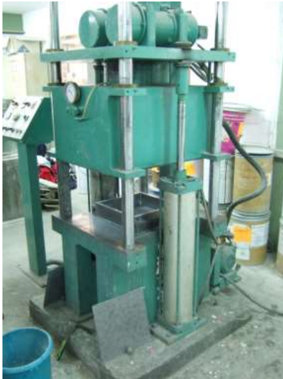
Fig. 8.1 Pilot plant for the analysis of the vibrocompaction process
