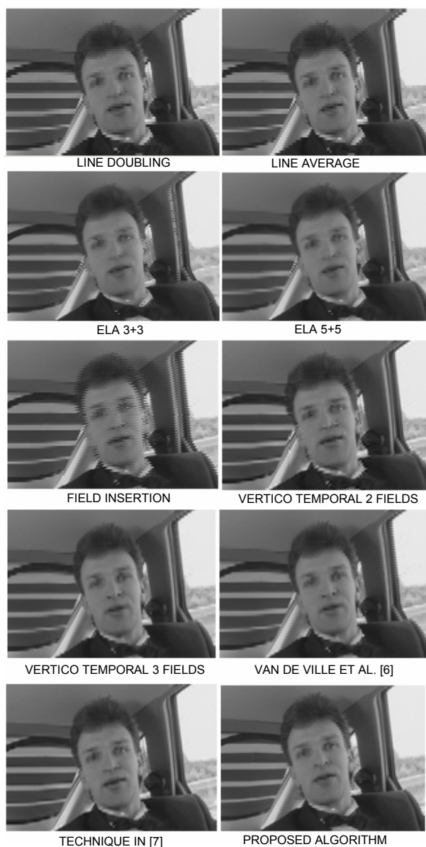
Figure 7: De-interlaced frames of Carphone sequence.
