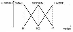
Figure 2: Membership functions for the fuzzy motion adaptive system
