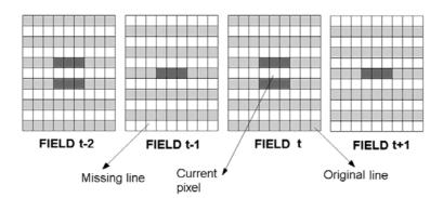
Figure 3: Pixels in dark grey are taking part in bi-dimensional convolution
