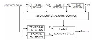
Figure 4: Block diagram of the fuzzy motion adaptive algorithm
