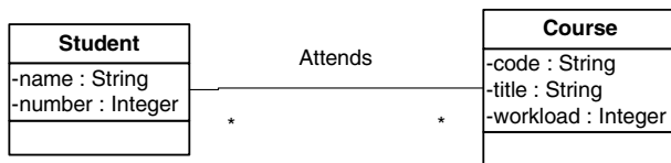
Fig. 15. Simple UML Diagram that shows a relationship between the students that attend some courses
