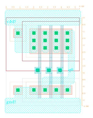
Fig. 3. Layout of the NOR-3 gate (UMC 0.18  $\mu$ m)
