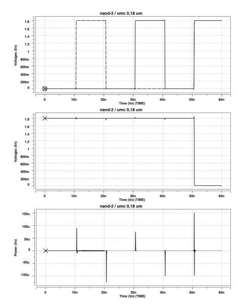
Fig. 6. Simulation detail of the NAND-2 gate (UMC 0.18  $\mu$ m): input signals (top), output signal (middle), and power dissipation (bottom)
