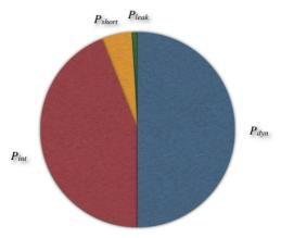
Fig. 1. Approximate contribution of the power sources to the total energy in a logic gate working at 50 MHz (0.18  $\mu$ m technology)
