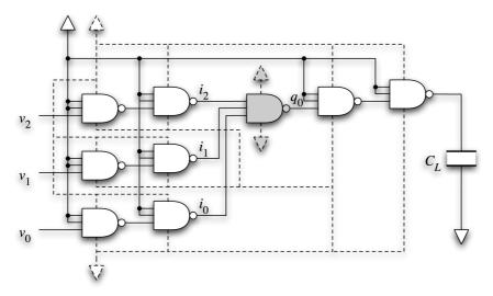
Fig. 4. Test circuit for the NAND-3 gate. The are two different power supplies (dashed): one for the device under test (shaded in gray) and another one for the rest of the gates.
