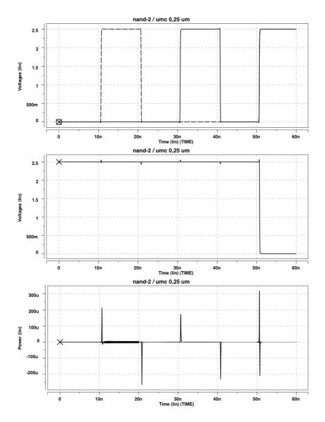
Fig. 5. Simulation detail of the NAND-2 gate (UMC 0.25  $\mu$ m): input signals (top), output signal (middle), and power dissipation (bottom)
