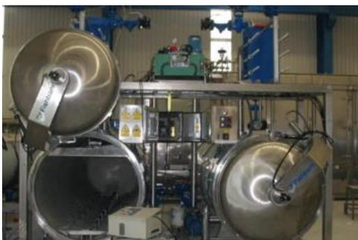
Figura 14: Autoclaves horizontales.
